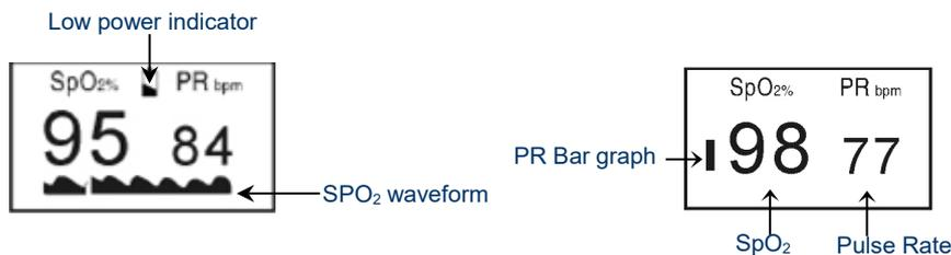
The PR Bar graph displays corresponding with the patient's pulse beat. The height of the bar graph shows the patient's pulse strength.
